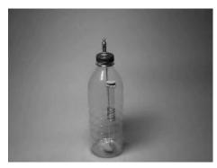
Figure 2. Plastic bottle with a test tube covered by a rubber membrane.
