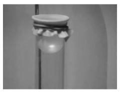
• Replace the rubber membrane with a thin plastic membrane. Under the influence of pressure it is also bent into a test tube (Figure 3). If overpressure in the bottle is sufficiently great, the plastic membrane ruptures (see Figure 4).
