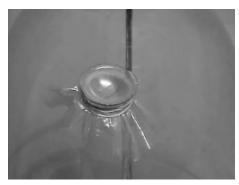
Figure 4. Plastic bottle with test tube covered by a ruptured plastic membrane.
